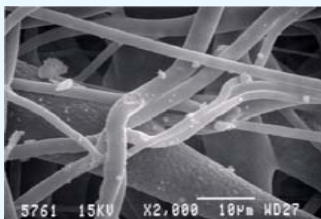
Figure 3: SEM micrograph of PU/PCL (75/25) mat containing ketoprofen before drug release.
